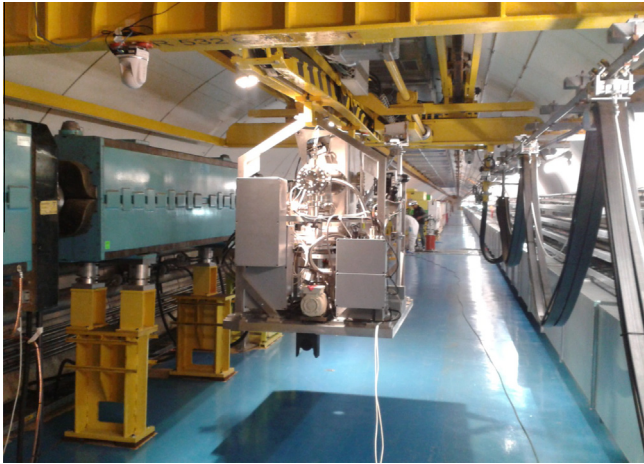
Fig. 7. Installation of the HRMT-14 test-bench showing HiRadMat tunnel and equipment.
